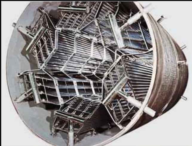
Banks in highly agitated polypropylene reactor
