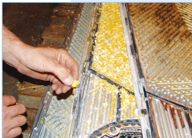
Plates and gaskets from other manufacturers are analyzed to determine if original specs still apply, and what cleaning procedures will be most effective.
