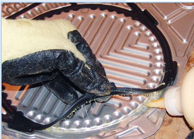
Plates are regasketed with OEM replacement gaskets, using a non-hardening, OEM-spec adhesive that does not require heat curing.
