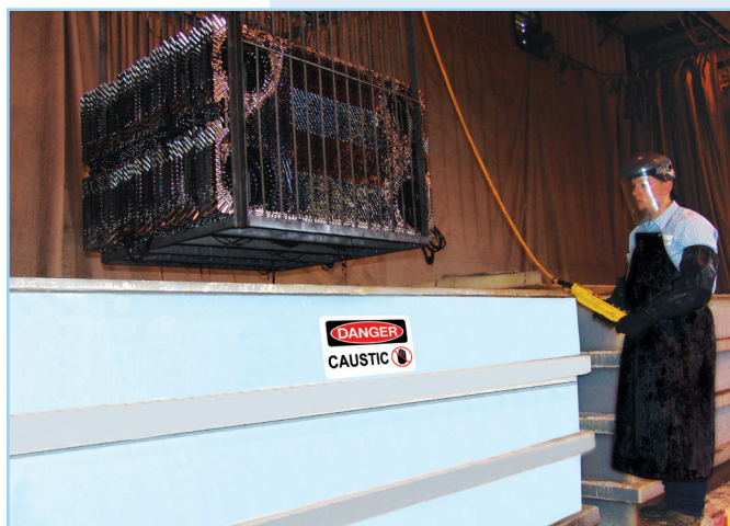
Plates are immersed in caustic and acid baths compatible with the plate material.
