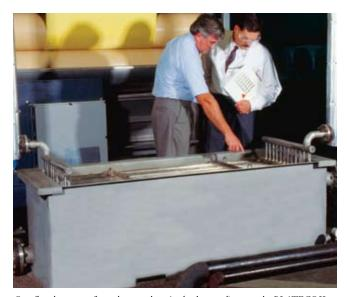
Overflow hot water from three washers (in background) enters the PLATECOIL bank at lower left at 90°C (195°F), then transfers heat to fresh water before exiting to an outside drain (bottom right) at 57°C (135°F).
