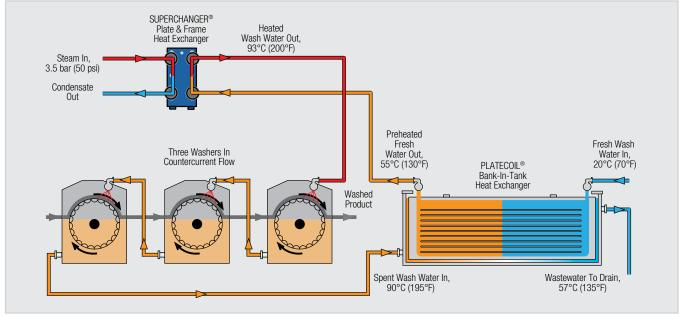
Countercurrent flow through the SUPERCHANGER® unit employed as a steam heater aids efficient heating of the preheated fresh water. The PLATECOIL bank-in-tank unit recovers heat from the particle-laded spent wash water with low maintanence.
